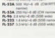
FL-52A 500 Hz-6 dB (CW/RTTY narrow)
