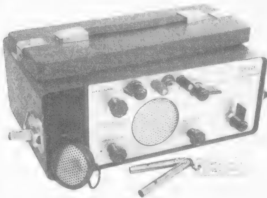
Figure 1. Type 6104 transceiver, Eilco's first set. Note the two whistles used to give the emergency tones
