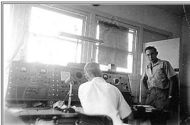
Leigh Creek Aeradio Control Console Including tunable AR7 Receiver
