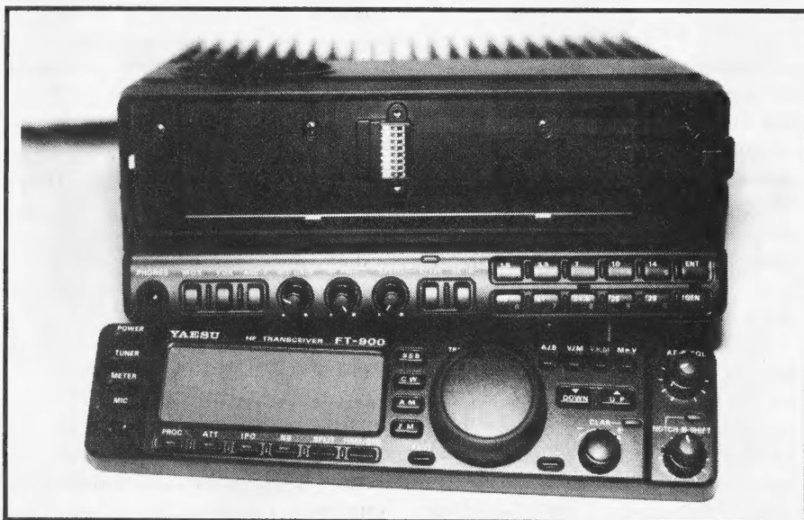
FT-900 transceiver with the front panel detached.
