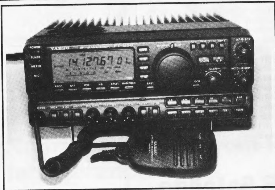
FT-900 transceiver with front panel attached, and HM-31 microphone.
