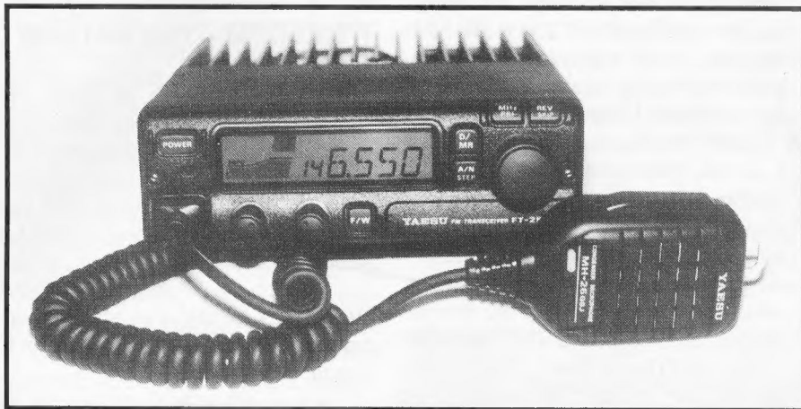
Front view of the FT-2500M with the matching MH-26G8J electret microphone.
