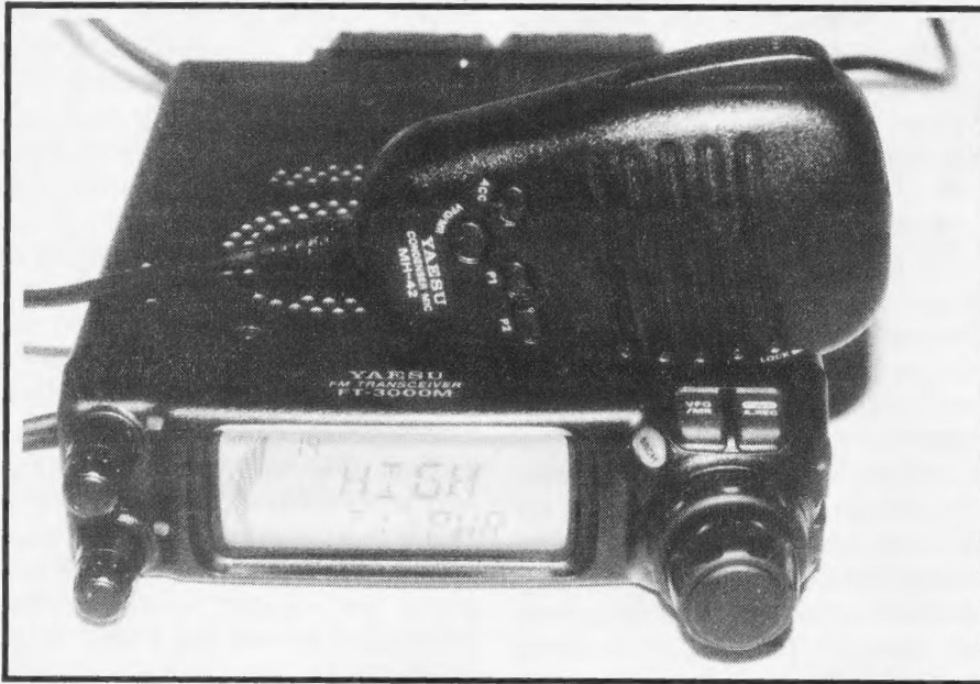
The Yaesu FT-3000M. Comparison with the microphone shows the compactness of this high power rig.
