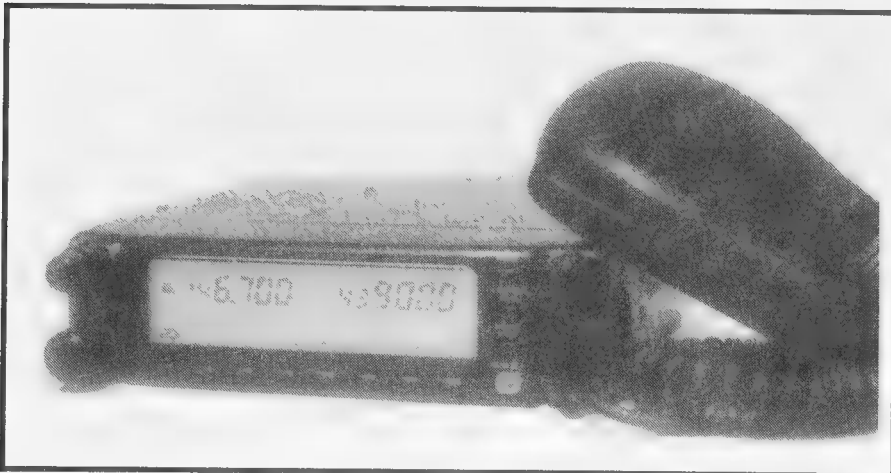
The Yaesu FT-8100R. Note the uncluttered front panel, and how compact the transceiver is in comparison to the standard-sized hand-held microphone. (Photo by Vicki VK3LT)
